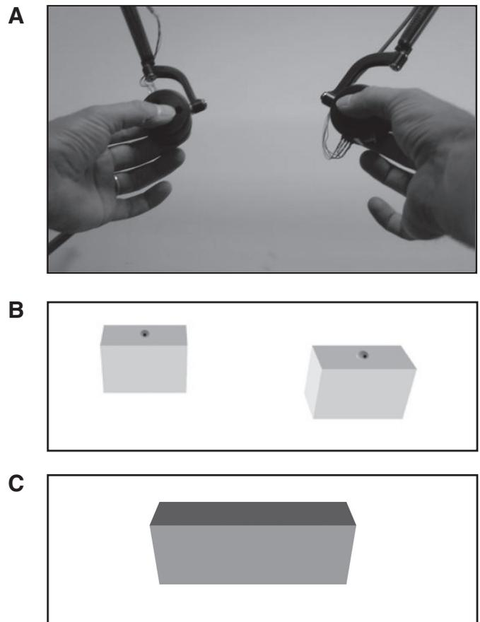
FIG. 1. Experimental apparatus. A: the participant held each grip force sensor attached to the robot arms with a precision grip (index finger opposing the thumb). During the experiment, the participants could see either 2 separate objects (B) or 1 object (C), and the corresponding object dynamics was simulated to calculate the forces produced by the robotic arm. The small spheres represent the location of the link between the object and the hand (hands not visible in C).
